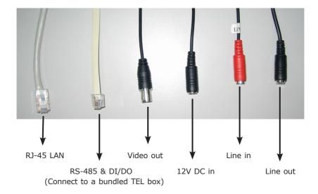
**1. RJ45 LAN socket:** Connect to PC or Hub/Switch. For connect to 10Base-T Ethernet or 100Base-TX Fast Ethernet cabling. This Ethernet port built N-Way protocol can detect or negotiate the transmission speed of the network automatically. Please use Category 5 "straight through" cable to connect the ICA-525 to a 100Mbps Fast Ethernet network switch or hub.
